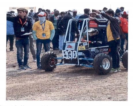
**Maneuverability test:** In this event vehicles steering is tested where it is made through pass through sharp corners and unsteer able paths. The vehicle which completes this path in shortest time is awarded.
